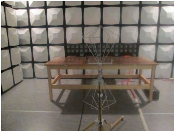
Fig. 2. Testing setup for chamber validation with biconic antenna in semi-anechoic room
