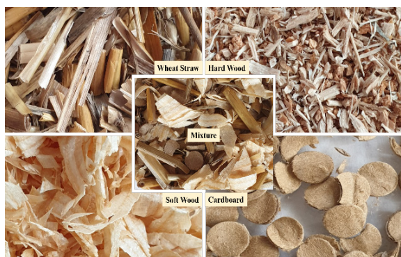
Figure 1. Types of lignocellulosic biomass (hard wood, soft wood, wheat straw, cardboard, mixture).
