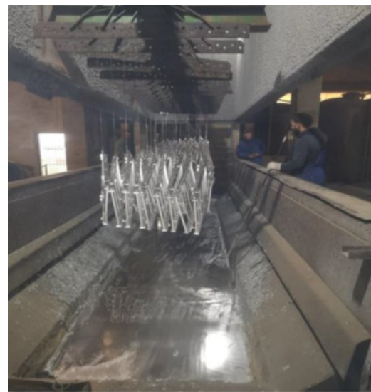
Fig.1 Retrieving parts from thermal galvanizing process
