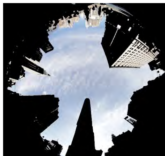
Segmentation result (the non sky region is colored in black) obtained applying an original segmentation method.
