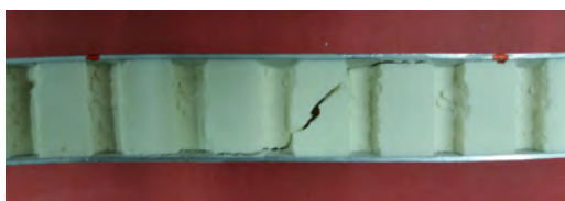
Fig. 4c. core fracture (PSP 2)
