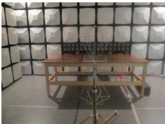
Fig. 2. Testing setup for chamber validation with biconic antenna
