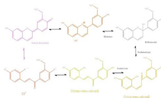
Fig. 2. The network of chemical reversible reactions of one of the dyes species upon pH changes
