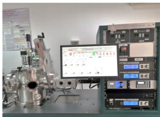
System for deposition of compositional spread libraries installed in Politehnica University Timisoara
