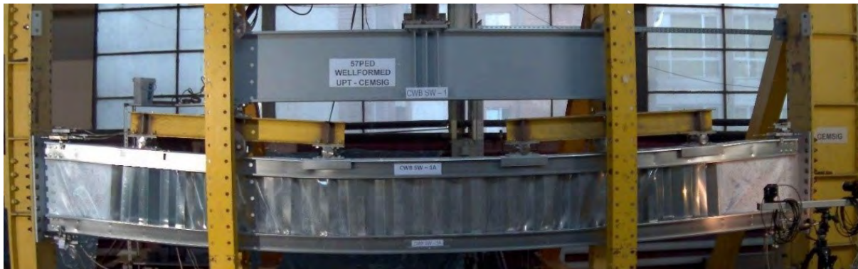
Fig. 2: SW1 CWB Beam during the test
