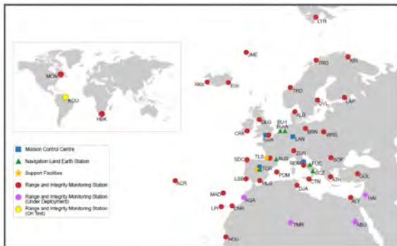
EGNOS Ranging and Integrity Monitoring Stations (RIMS) Sites
