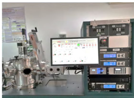
Fig. 1. System for deposition of compositional spread libraries installed in Politehnica University Timisoara
