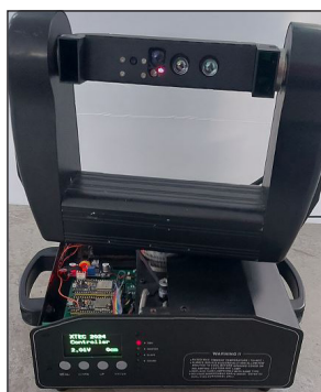
Fig.2. Optical Tracking: Integrated a Jetson Xavier edge-AI platform capable of real-time bounding-box detection and “Slew-to-Cue” camera orientation
